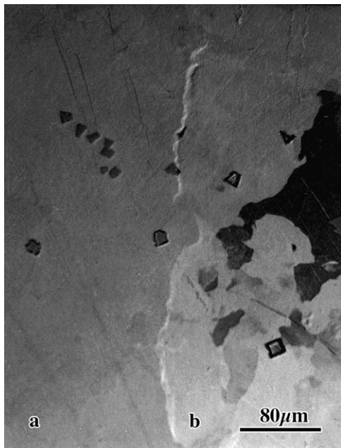
Fig. 1. An as-cast uranium sample which has been final polished (a) on medium nap cloth (Microcloth) using 1 \mu\text{m} diamond abrasive with a propylene glycol lubricant for \sim 10 min, followed by (b) electro-polishing using a 5% \text{H}_3\text{PO}_4 solution at 3 V for \sim 2 –3 s. After mechanical polishing, the sample was masked with tape on the left side and then electro-polished. The sample was photographed using differential interference contrast (DIC).
