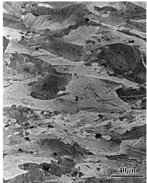
Fig. 5. DIC light micrograph of warm rolled uranium (275 °C), subsequently annealed at 450 °C for 1 h, showing a partially recrystallized structure. The sample was electro-polished with 5% \text{H}_3\text{PO}_4 at 3 V for \sim 4 s.
